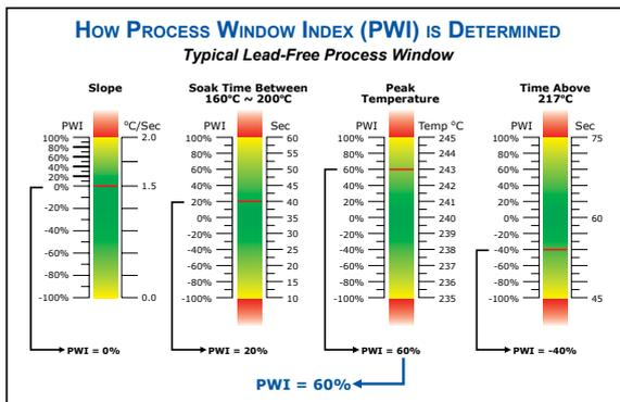
The Process Window Index is calculated using a formula that includes all statistics for all thermocouples.
