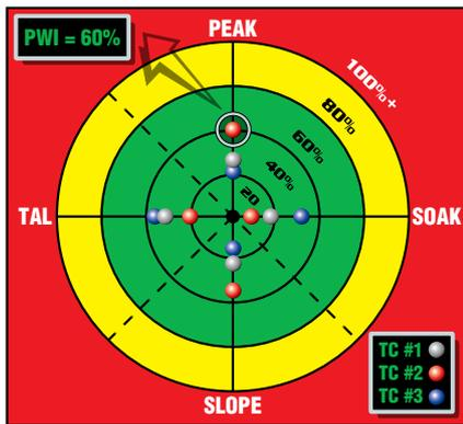
The Process Window Index for a complete set of profile statistics is calculated as the worst case (highest number) in the set of statistics. For example: if you run a profile with three thermocouples, and four profile statistics are logged for each thermocouple, then there will be a set of twelve statistics for that profile. The PWI will be the worst case (highest number expressed as a percentage) in that set of profile statistics.
