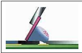
Fig. 7. This picture is taken from an animation in PasteMaster®. The animation is based on a study with high-speed video recordings of aperture filling. It clearly shows the backfill effect when the paste flows into the aperture.
